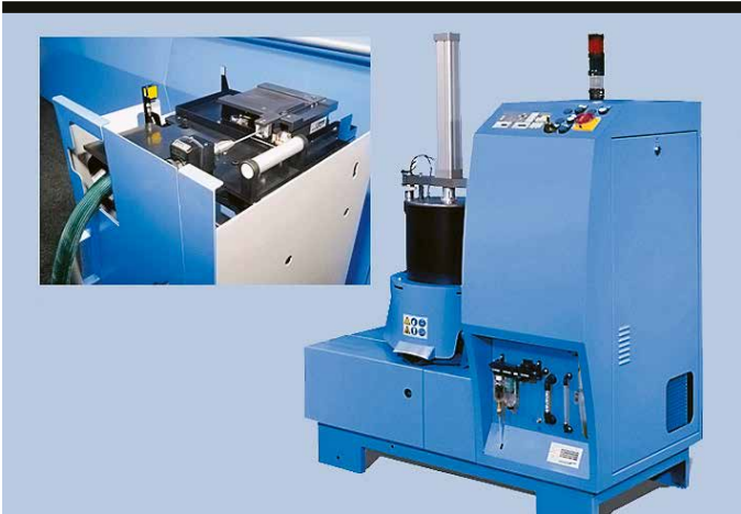
Softcover production: retrofit for PUR spine gluing
