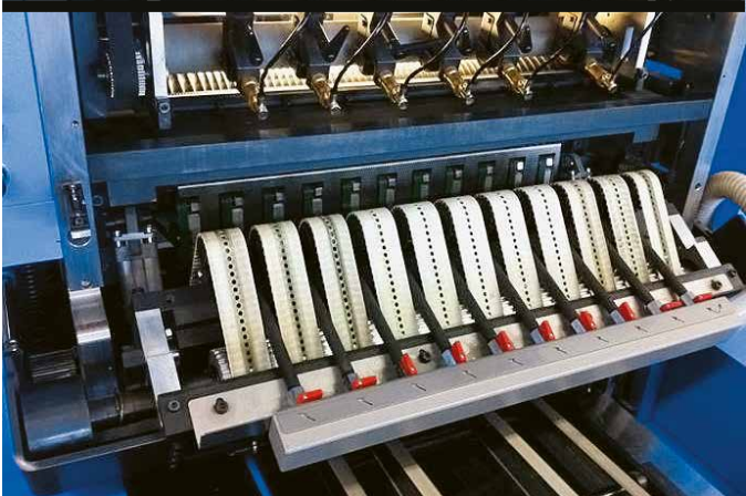
Digital solutions: vacuum transport for the cross fold
